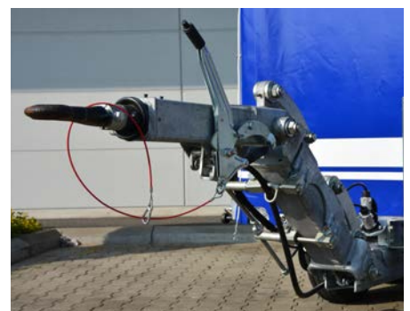
Drawbar that can be adjusted in height
