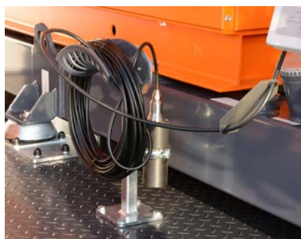
Automatic operation via level sensor
