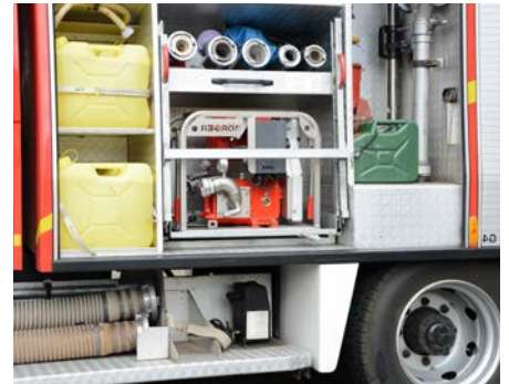
With a combustion motor, the pump can be carried by four persons
