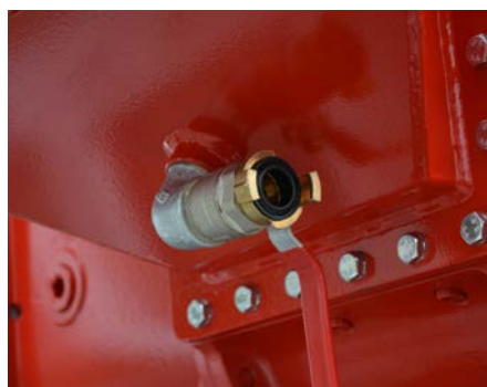
Drain for removal of residues
